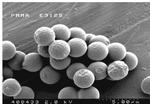
Figure 2. SEM images of PMMA particles prepared with Krytox 157FSL (1 wt % wrt MMA).
